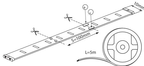
$L = 5\text{m} (50 \times 100\text{mm}) = 150\text{LED}$
