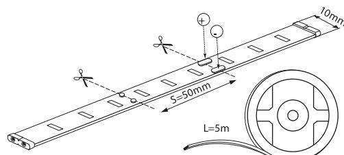
$L = 5\text{m} (100 \times 50\text{mm}) = 300\text{LED}$
